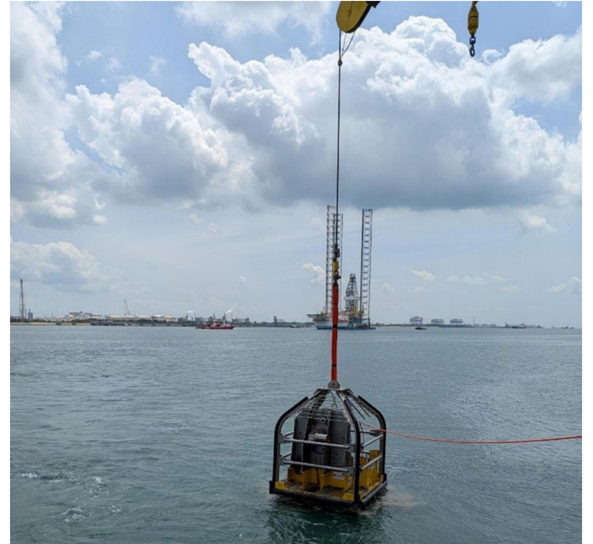
Figure 3: Deployment of Cone Penetrometer Testing (CPT) equipment, used to assess the soil properties and strength of the seabed for subsea cable installation.
