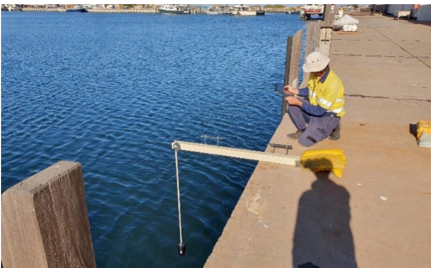
Figure 3: Specialist scanning rig; offers mobile and lightweight scanning tool close to the jetty; enabling accurate point cloud data to be captured over short distances under for low freeboard or limited access marine structures
