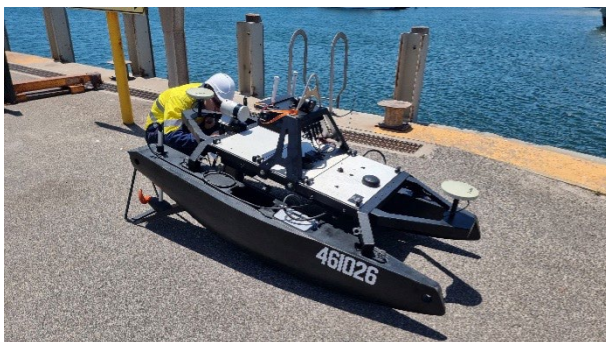
Figure 7: Unmanned Surface Vehicle; with lower freeboard and size compared to conventional survey vessels; offering greater versatility for surveying in tight locations
