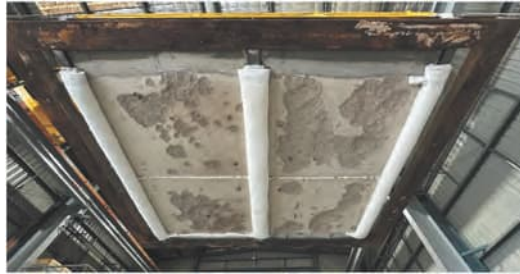
Figure 3. View of the test specimens after fire test whilst in the frame holder.
