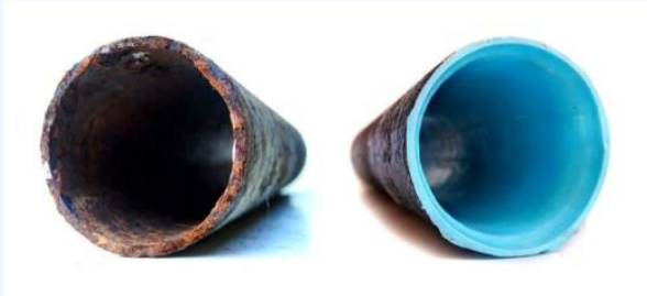
Epoxy Pipe Lining
