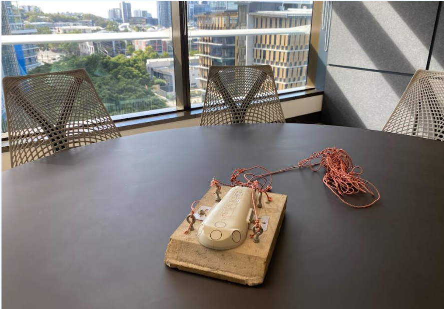
SonTek IQ+ and Concrete Anchoring Block
