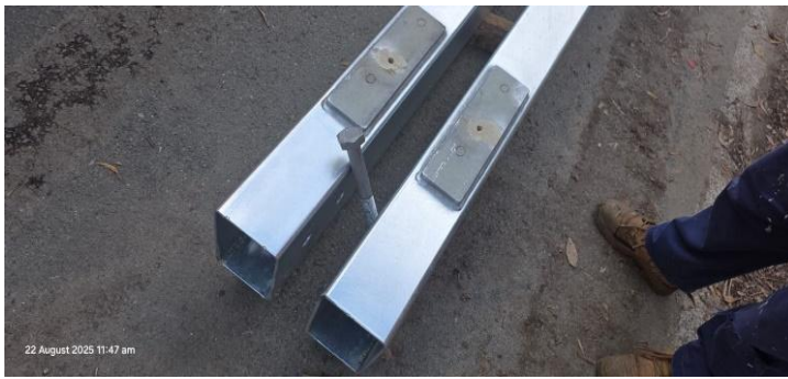
Figure 15. Bolt unable to be put through hole in barrier
